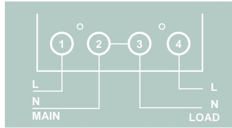
*Check that the rotation is left to right. If not-rewire correctly.*
