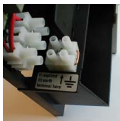
Fit earth terminal as shown if required
