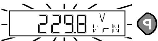
Scrolling through Page 3 with the *down* button brings up the display for red to neutral voltage, as this is the first item within that page. Press the *left* button to add this to the Favourites Page. The display then stops flashing.
