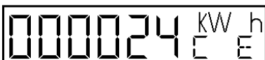
Cumulative total register for kWh export, in this case showing 24 kWh. (Only on model EN305).
