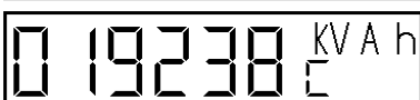
Cumulative total register for kVAh, in this case showing 19238 kVAh. Measurements of apparent energy and demand are active in all four quadrants. (Only on model EN305).
