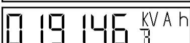
Billing register for kVAh, in this case showing 19146 kVAh. (Only on model EN305).
