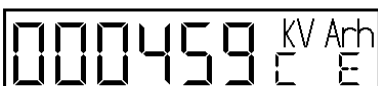
Cumulative total register for kvarh lead, in this case showing 459 kvarh. (Only on model EN305).
