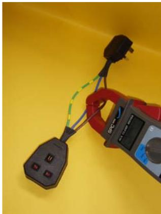
**NOTE:** Clipping the unit around the live and neutral conductors together will not work. The *SPCMini* must be clipped around the live cable only.
