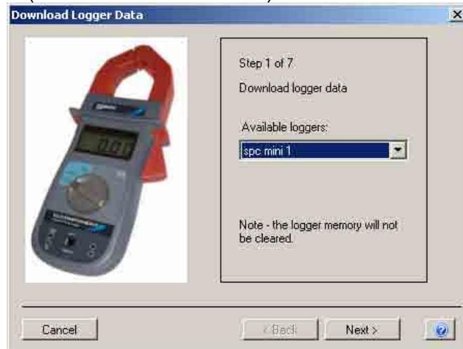
Check that the logger shown in the 'available loggers' window matches the logger you wish to download, or select an alternative if multiple loggers are available.
