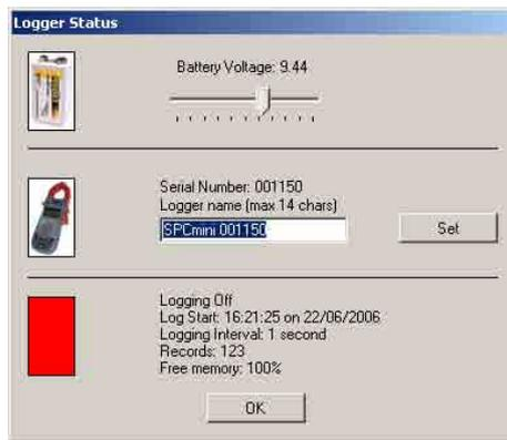
Battery Voltage should read over 7.5V. If the reading is lower than this, replace the battery.
